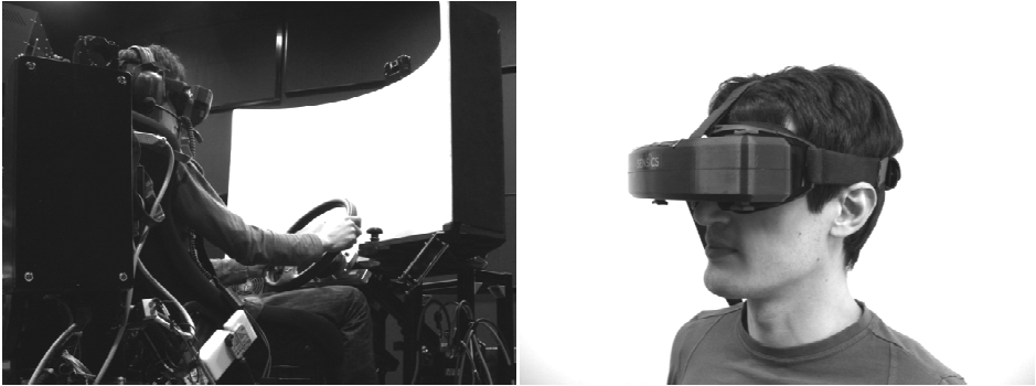
Figure 2. (a) The projection screen mounted to the CyberMotion Simulator; (b) the Sensics xSight HMD. The optics for both eyes can be moved sidewise to match the user's anatomy
