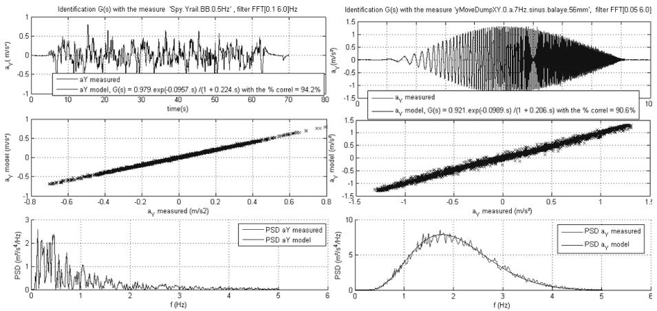
**Figure 1. Example of identification output signal (top), comparison of model predictions vs. measurements (middle), and acceleration spectral distribution (bottom), for a pseudo-white noise (left) and swept sine (right)**
