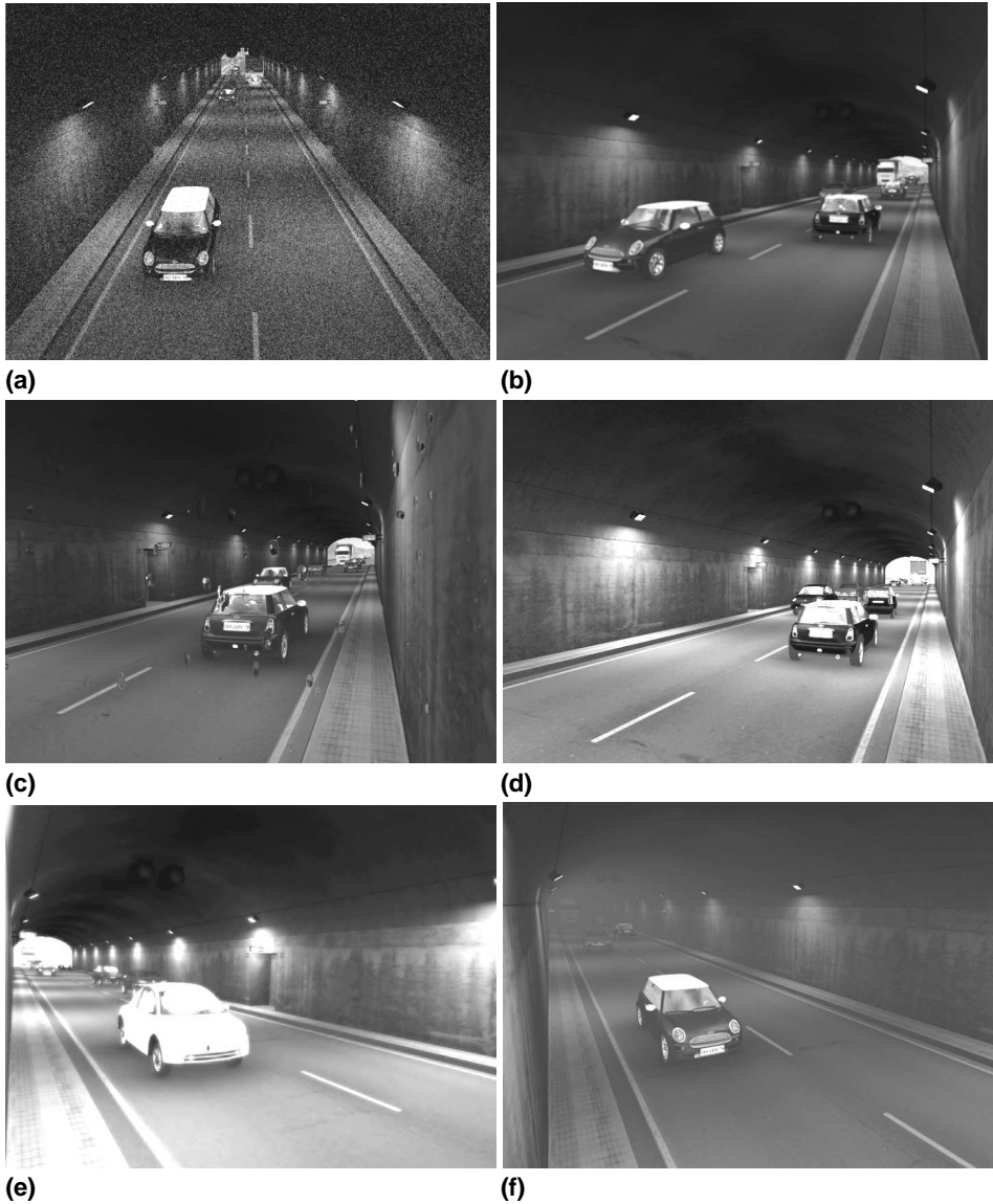
Figure 5. Multi-rendering and filters mechanism: a) Noise, b) Depth of field, c) Color, d) Rain drop, e) Auto exposure, f) Fog
