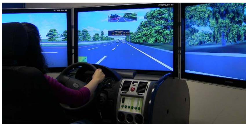
Fig. 1. VMS simulation with the driving simulator.
