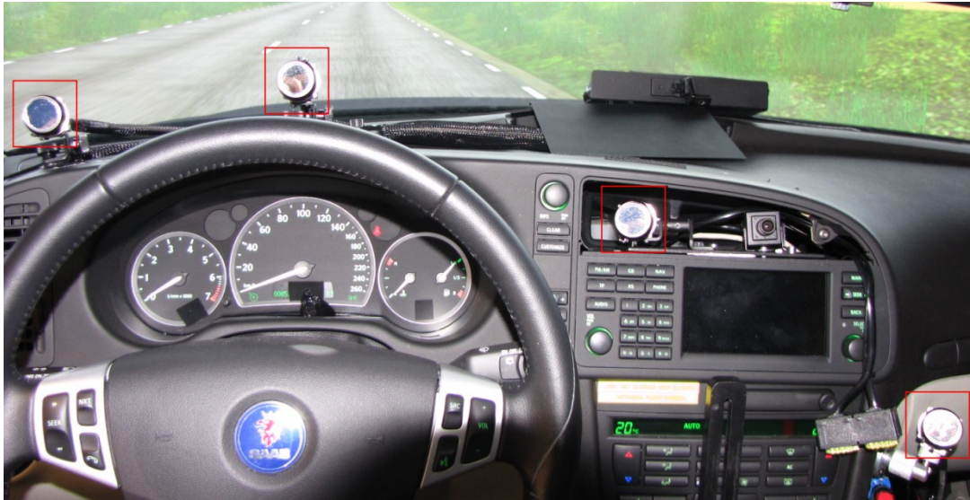
Figure 2. Camera placement in simulator cabin. Cameras highlighted by red markers.
