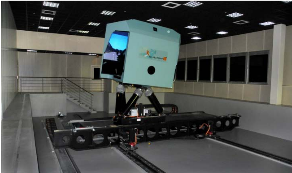
Fig. 1. PSA Peugeot Citroën's dynamic driving simulator SHERPA 2 .
