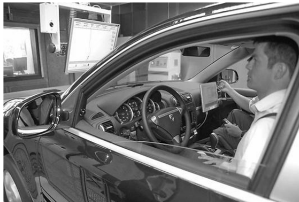
Fig. 3. The NEDC performed on a roller test bench with a monitor showing the target speed [FOC1]
