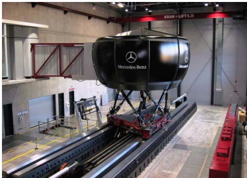
Fig. 1. Moving base simulator (Daimler AG).
