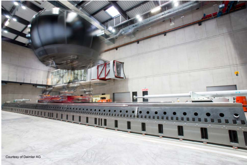
Fig. 1. The motion system of the Daimler driving simulator.
