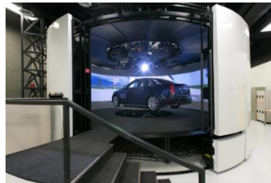
Fig. 1. Driving simulator (access door in cab exchange position).
