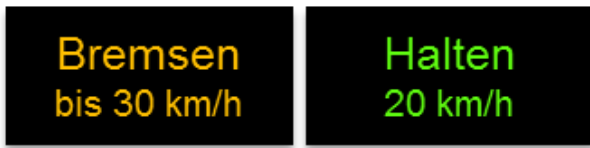
Figure 2: examples for recommendations of the traffic light assistant in the HMI (on the left: slow down to 30 km/h ; on the right: drive 20 km/h).
