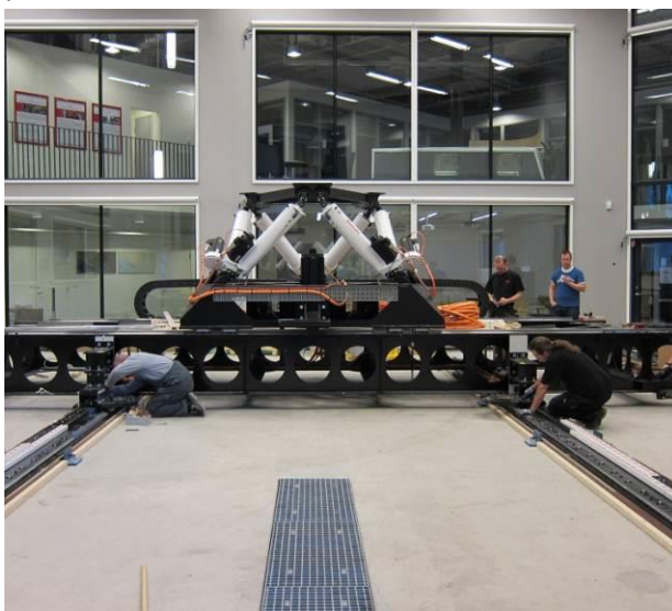
Figure 4. The moving base of Sim IV consist of a bi directional large stroke linear system and a hexapod. In this case a commercial solution that has been deployed in several other advanced driving simulators.
