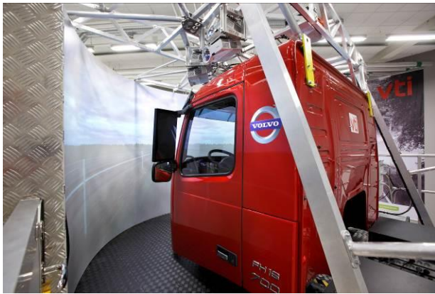
Figure 3. This picture show the beam connecting the back corner of the cabin to the platform structure.
