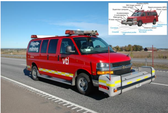
Figure 1. The VTI Road Surface Tester measurement van with its front mounted laser interferometer array.
